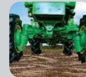
4 wheel drive with Heavy Duty Front Axle
