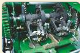
Standard Knotter Set (Deering Type) with cleaning fan Uniform and smooth binding of bales
