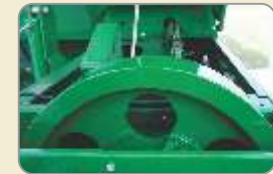
Balanced flywheel with counter weight & powerful gear box Smooth operation and more stability
