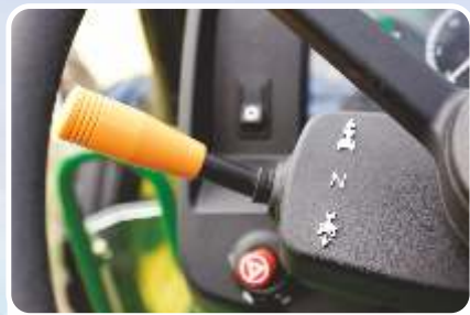
Forward - Reverse tractor without operating clutch and gear
